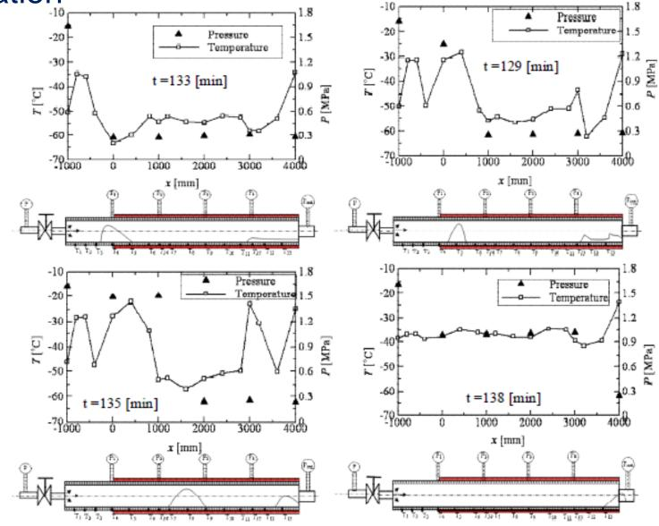
Variations of local pressure and wall temperature with the dry ice sedimentation inside the test section at different times
