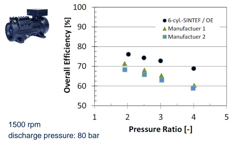
superheat at the compressor inlet: 10 K
