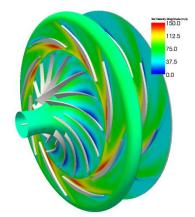
CO<sub>2</sub> turbo compressor Reference: Hafner et al 2011
