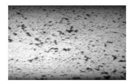
(a)  $CO_2$  solid-gas flow at opening conditions of 15mm of expansion value
